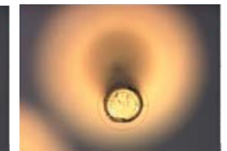
Circle probe appears on the abnormal pin location without measurement failure
